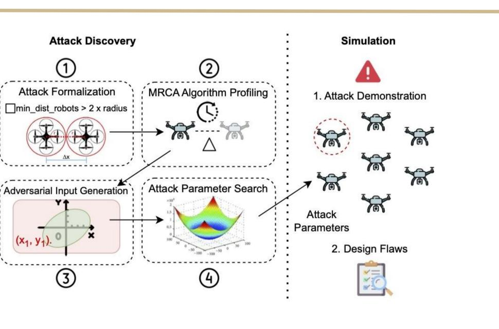
Successfully identified semantic attacks against ORCA and GLAS algorithms. Demonstrated stealthiness by evading anomaly detection mechanisms. Conducted experiments using high-fidelity simulator and Crazyflie drones demonstrating practicality of attacks.
